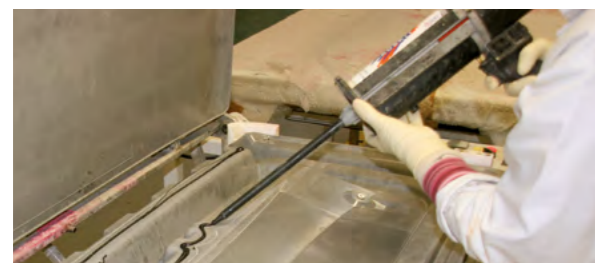
Bonding of SMC parts with Adekit A280.
